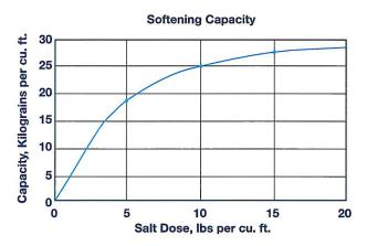
Capacity and leakage data are based on the following: 2:1 Ca:Mg ratio, 500 ppm TDS as CaCO<sub>31</sub> 0.2% hardness in the salt and 10% brine concentration applied co-currently through the resin over 30 minutes. No engineering downgrade has been applied.
